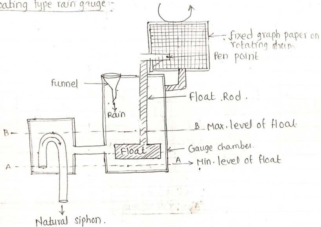
→ Rotating drum - A rotating drum consist of graph paper fixed around it. A pen point which is in contact with graph paper moves up with the rise of float. The rain water enters through funnel gets collected in gauge chamber. When the chamber get filled up to level B-B a natural siphon starts working & rain water is drained out. At the same time float moves downward & process continues.
