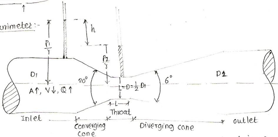
By decreasing area of throat, velocity & hence velocity head increases. This increased vel. head reduces pressure head ( $\frac{P_2}{\gamma}$ ) at throat section.
