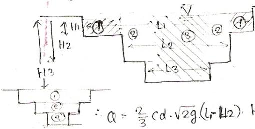
stepped notch is a combination of rectangular notches. This notch is useful for measuring accurate discharge at low & high head.
