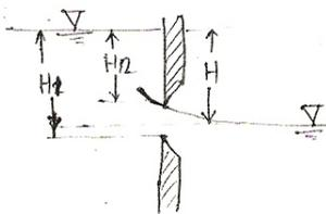
$$Q = \frac{2}{3} C_{d1} \cdot b \sqrt{2g} [H^{3/2} - H_2^{3/2}] + C_{d2} \cdot b \cdot (H_1 - H) \sqrt{2gH}$$
