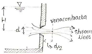
Venacontracta is a section of jet where stream lines are parallel to each other & far to the plane of orifice. The velocity of each particle is in the direction far to the plane of orifice.
