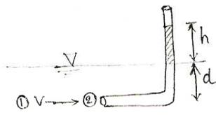
To measure vel. of flow in open channel, pitot tube is immersed in water. Due to vel. of flow water level rises by 'h' in pitot tube
