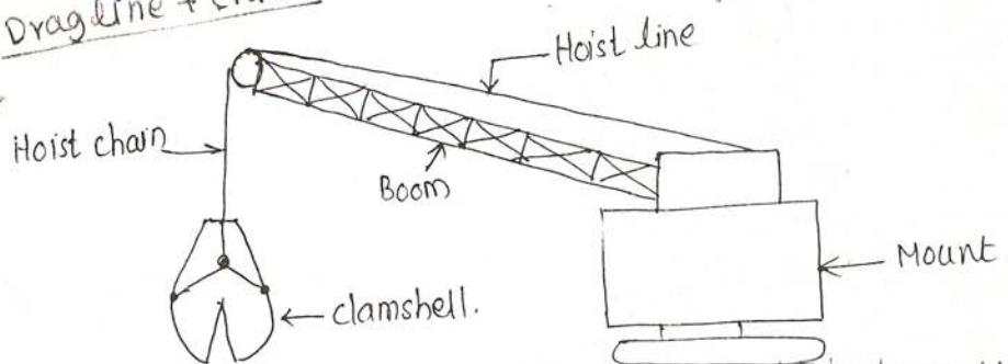
Use: Handling loose matl. like sand, gravel, crushed stone, coal. Removing matl. from coffer dam, pier foundation, sewer manholes. Vertical lifting.
