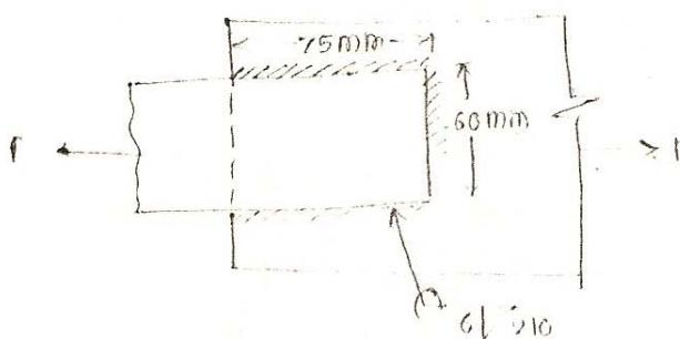
Soln:- Eff. length of weld =  $75 + 60 + 75 = 210\text{ mm}$ .
