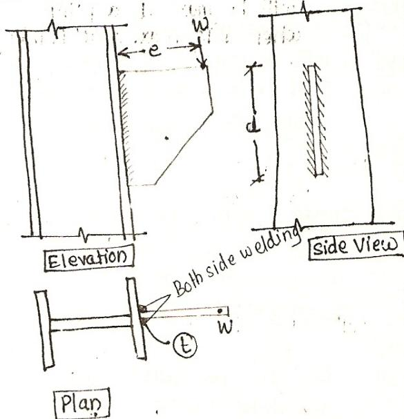
Consider a bracket connection to the flange of colm by a fillet weld as shown in fig.
