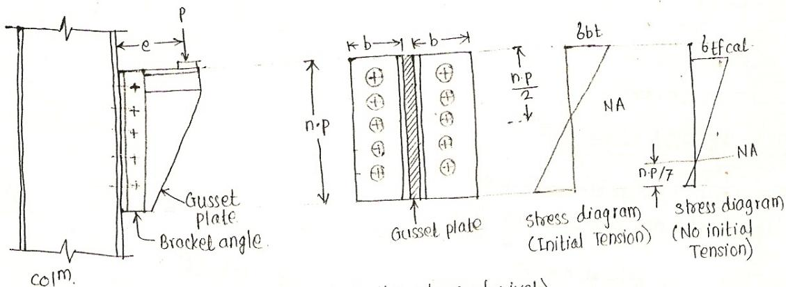
Bracket type II (Moment is not in the plane of rivet)
