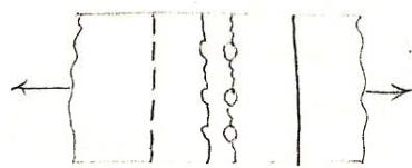
reduced by rivet holes & the plates may tear off along the line of rivet holes.
