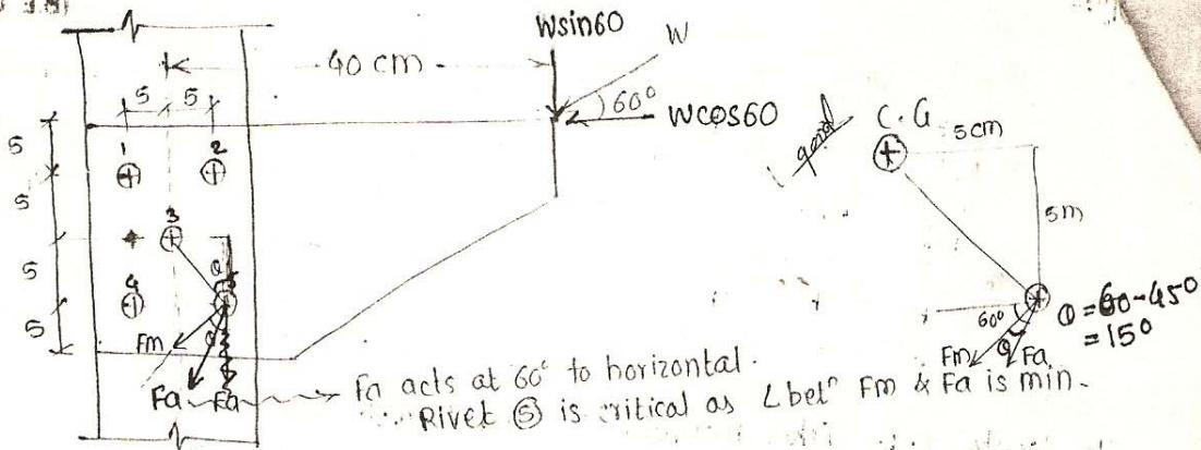
Sol<sup>n</sup>:- Due to symmetry C.G. of rivet group is at rivet 3.
