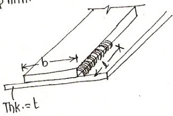
④ Intermittent fillet weld :- Intermittent fillet weld may be used when the length of smallest size fillet weld reqd. to transmit stress is less than the continuous length of joint.
