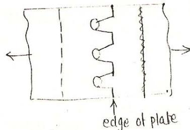
The plate will crack at the back of rivet if it is placed very near to edge of plate. This failure is prevented by keeping min. edge dist.
