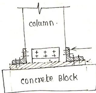
Size = 75x75x8, Min. dia. of Rivet = 16 mm
