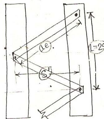
\* Design of lacing: single lacing system inclined at  $45^\circ$  with axis of col<sup>m</sup>. (o)
