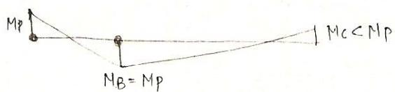
On further increase in load, plastic sectn at A rotates without absorbing any more mmt. The M<sub>B</sub> increases till it reaches to M<sub>p</sub>, & then plastic hinge is formed at B.
