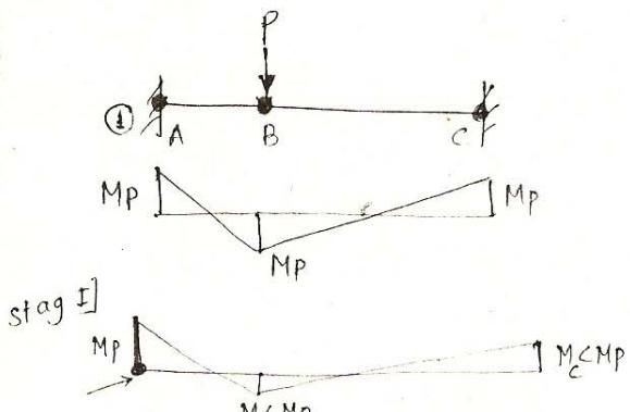
As load increases, the beam reaches its elastic limit at end 'A' & plastic hinge is formed. The mmt at B & C are less than plastic mmt.
