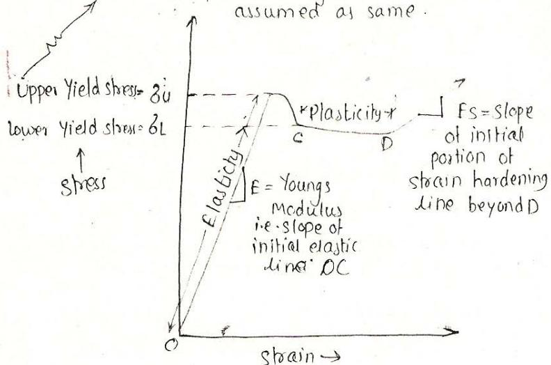
Enlarged Stress-strain Curve.
