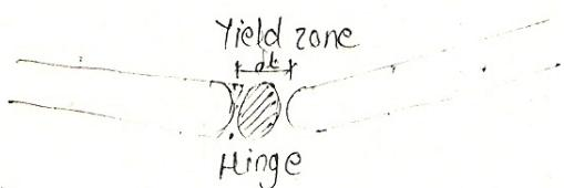
As the value of moment adjacent to yield zone is more than yield mmt, up to certain length depending upon loading & geometry of sect<sup>n</sup>; but for simplicity it is neglected. But it can not be neglected for calculation of deflections & design of bracings.
