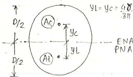
$$y_L = y_C = \frac{4D}{3\pi} = \frac{2D}{3\pi} f = \frac{Z_p}{Ze} = \frac{[A_c \cdot y_c + A_t \cdot y_L]}{\frac{\pi/64 \cdot D^4}{y_{max}}} = \frac{[\frac{\pi}{8} D^2 \times \frac{2D}{3\pi} + \frac{\pi}{8} D^2 \times \frac{2D}{3\pi}]}{\frac{\pi}{64} \cdot D^4}$$
