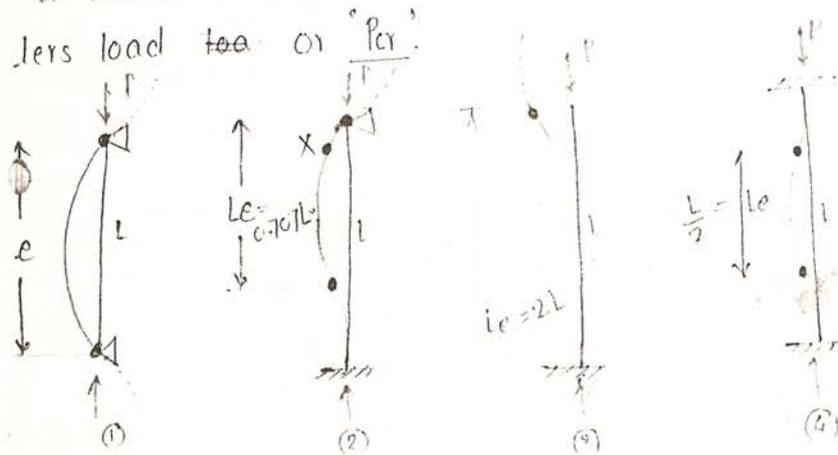
$$P_{cr} = \text{Buckling load} = \frac{\pi^2 EI}{(L_e)^2}$$
