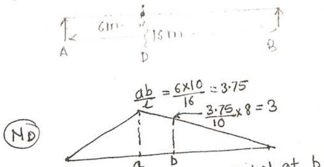
⑤ ∵ place 200kN at a, 80kN at b
