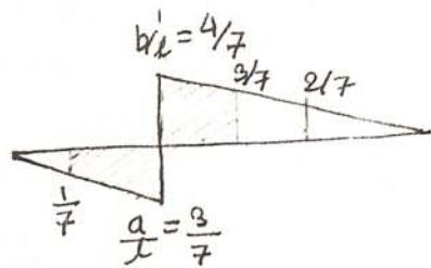
$$\therefore V_x = - \left[ \frac{1}{7} + \frac{3}{7} \right] \times \frac{2}{2} \times 80 + \left[ \frac{4}{7} + \frac{3}{7} \right] \times \frac{1}{2} \times 80 + \frac{2}{7} \times 90 \\ = +20 \text{ kN.}$$
