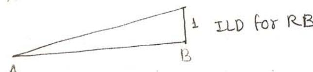
ILD for shear force at a section:-
