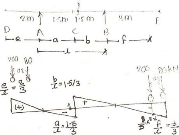
$$\therefore \text{for } -\text{SFmax} : -80 \times \frac{3}{5} - 200 \times \frac{1}{3} \times 2 = -181.333 \text{ kN}$$
